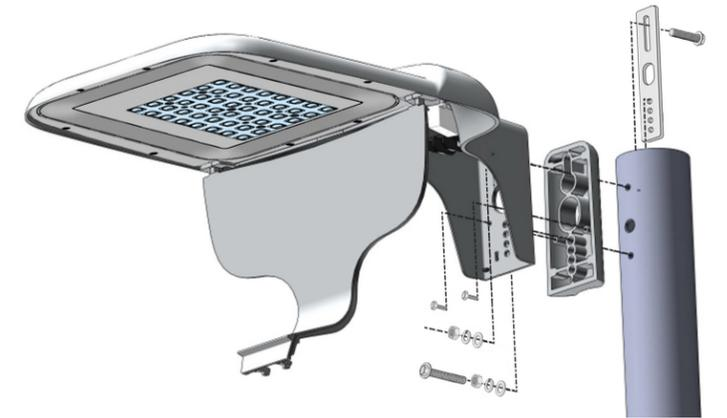
Arieta® easily mounts to square or round poles. Round Pole Adapter (RPA) required for round poles, as shown.
