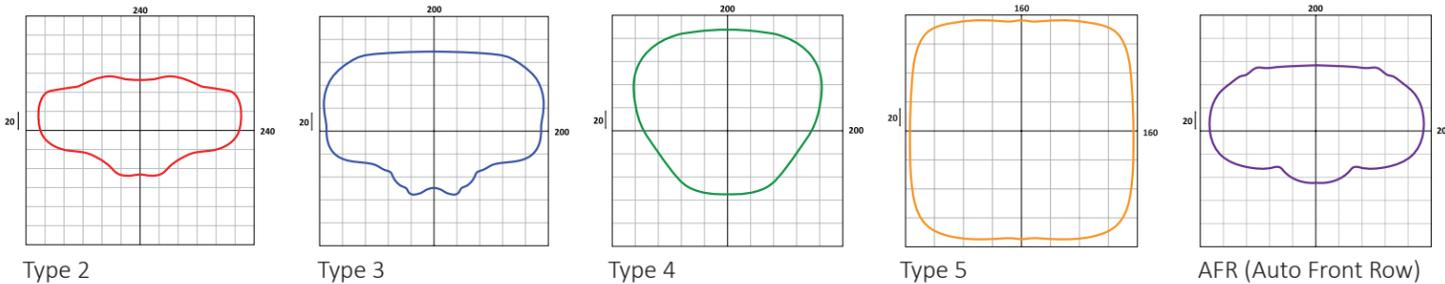
Micro-lens Optics produce IES Type 2, Type 3, Type 4, Type 5 distributions for Roadway and Area lighting applications. Factory rotated optics can be ordered for special applications.
